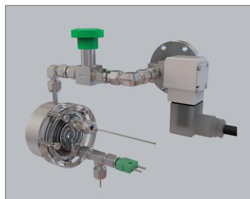
**Flow through probe** – circular carrier type inlet, with liquid flow connections. Includes the X44 membrane selected for high sensitivity to rare earth gases such as in ground water studies. A thermocouple and signal conditioning module are included for simultaneous acquisition and display of real time measured sample temperature data with mass spectrometer data.
