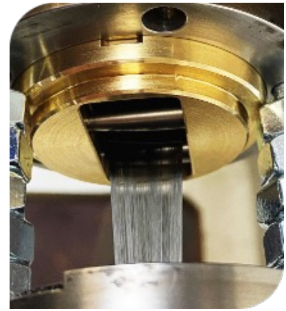
b.) spreaded fibers exiting the TOW impregnation die
