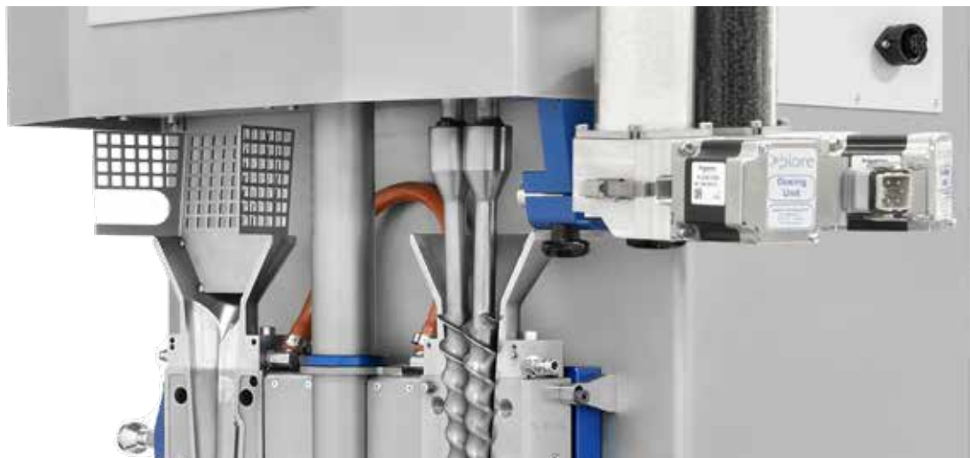
Figure 2. Xplore's microcompounder https://www.xplore-together.com/products/micro-compounders
