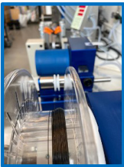
Optimum impregnation conditions: - 260°C – Moderate speed
