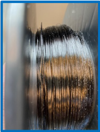
Optimum impregnation conditions: - 260°C – Moderate speed
