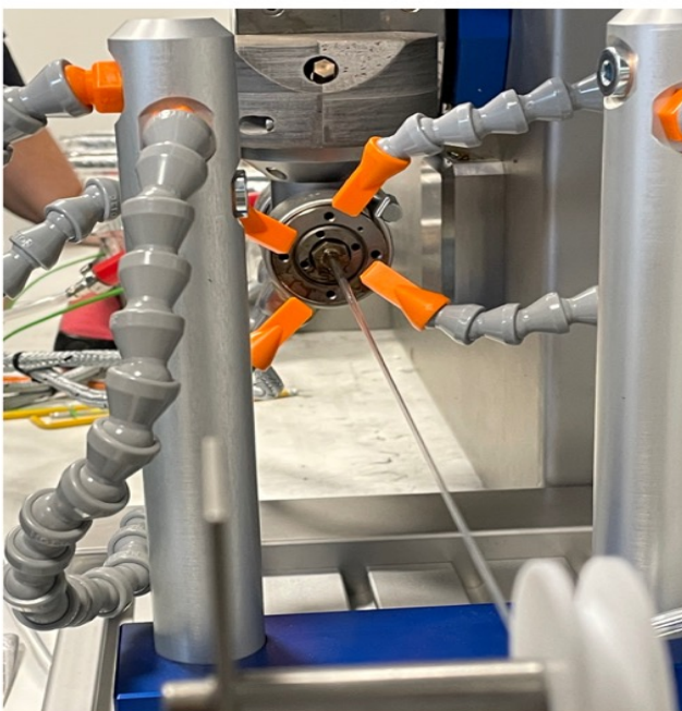
Figure 1. The micro-tube die attached to an MC 15 HT
